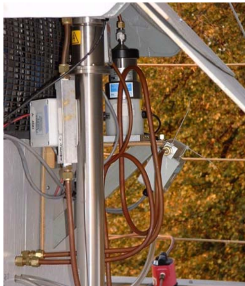
Detail of DMA Columns of DAASS, Deployed Outside of Enclosure to Reach Ambient Temperature
