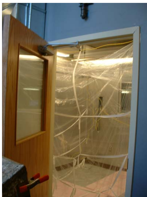
Teflon Bag Hanging inside the HVAC Controlled Enclosure
