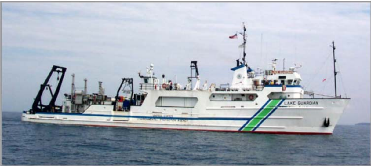
Figure 5. RV Lake Guardian. 180 feet; 850 ton displacement. Source: http://oceanexplorer.noaa.gov/technology/vessels/lakeguardian/lakeguardian.html
