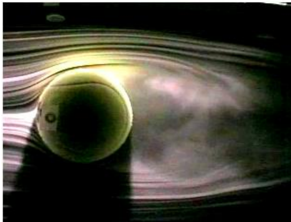
Conditions Producing Separation
