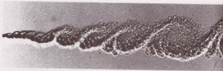
Fig. 5.51. A visualization of the flow of a plane mixing layer. A spark shadow graph of a mixing layer between helium (upper) U_h = 10.1 \text{ m s}^{-1} and nitrogen (lower) U_l = 3.8 \text{ m s}^{-1} at a pressure of 8 atm. (From Brown and Roshko (1974).)
