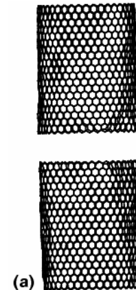
Fig. 23 Fracture modes of (a) a (40,0) zigzag nanotube with an initial crack of length 0.48 nm (Mode I fracture); (b) a (23,23) armchair nanotube with an initial crack of length 0.48nm (Mode I fracture); (c) a (23,23) armchair nanotube with an initial crack of length 0.92nm (Mixed Mode I/II fracture).
