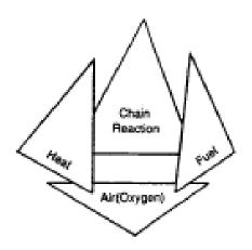
No fire can start or maintain itself unless all elements of the Fire Triangle or Fire Tetrahedron are present, i.e., fuel, oxidant, heat or spark, and free radicals. To avoid fires, control ignition sources, i.e., sparks, flames, static electricity, heat, friction, smoking, electric motors, etc.
