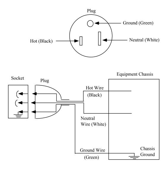
Figure II-2. Standard three-wire grounded wiring connection for 110-V electric power (adapted from *Prudent Practices in the Laboratory. Handling and Disposal of Chemicals*, National Academy Press, Washington, DC, 1995).
