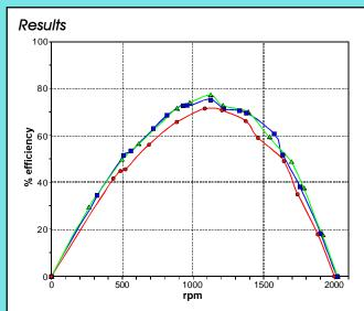
Results for three tests conducted at free-rotational speed of 2000 rpm. Under ideal conditions the maximum efficiency of the turbine isabout 85%
