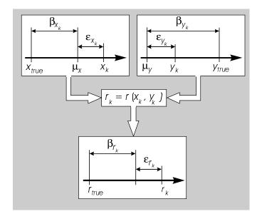
Figure 6. Propagation of bias and precision errors into a two variable result (Coleman and Steele, 1995)
