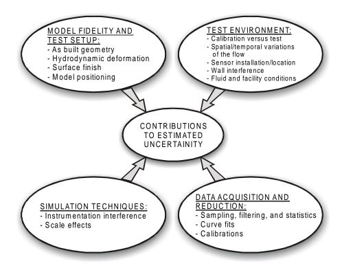
Figure 4. Sources of errors (adapted AIAA, 1995)
