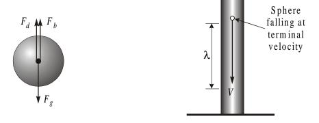
Figure 7. Experimental arrangement
