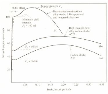
Figure 2.1.1 Typical stress-strain curves.
