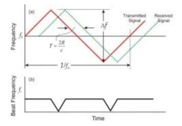
In the figure, (a) is the frequency-time relationship of an FM-CW radar with triangular modulation. The received signal (dashed line) from a target at range R is delayed a time T=2R/c.  $\Delta f$  is the frequency excursion and  $f_m$  is the modulation frequency. In (b) is the difference (beat) frequency between the transmitted and received signals. One can show that for a stationary target:
