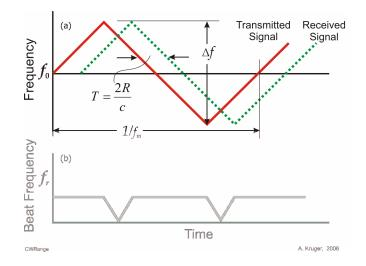
In the figure, (a) is the frequency-time relationship of an FM-CW radar with triangular modulation. The received signal (dashed line) from a target at range *R* is delayed a time T=2R/c.  $\Delta f$  is the frequency excursion and  $f_m$  is the modulation frequency. In (b) is the difference (beat) frequency between the transmitted and received signals. One can show that for a stationary target:
