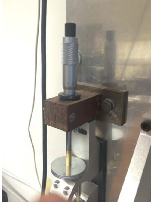
Figure 3: Final calibration setup with micrometer and sensor
