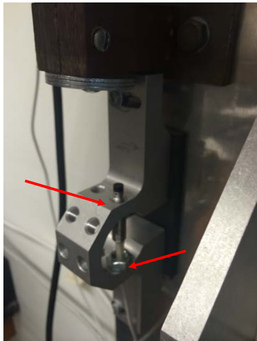
Figure 2: Inserting the induction sensor plug-end into the calibration setup
