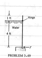
3.69 A rectangular gate is hinged at the water-line, as shown. The gate is 4 ft high and 10 ft wide. The specific weight of water is 62.4 lbf/ft<sup>3</sup>. Find the necessary force (in lbf) applied at the bottom of the gate to keep it closed.
