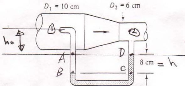
$$\text{Continuity: } A_1 V_1 = A_2 V_2 = Q \quad 2\frac{1}{3}$$
