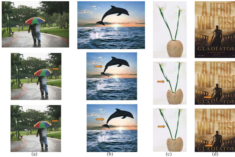
Figure 9. Image resizing using graph search method. The first row is the original image. The second row is the graph search result without the shape prior penalty. The third row is the result with the convex shape prior penalties. Typical improvements are pointed out by arrows.
