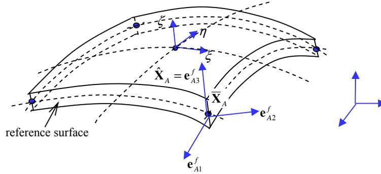
Figure 2: Geometrical description of the shell element
