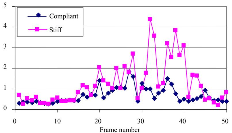
Fig. 10. Computed joint torques about the right knee exerted by the clothing.
