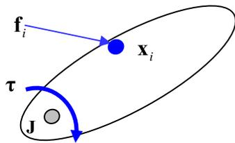
Fig. 9. Computation of instantaneous torques exerted by the clothing about the joint centers.
