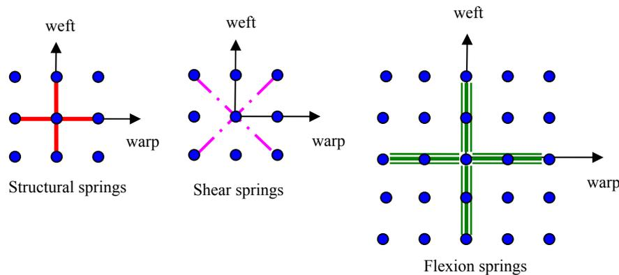
Figure 1: A mass-spring model by Provat
