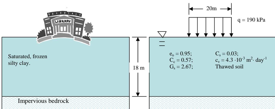
$$\Delta\sigma_v = q \left\{ 1 - \left[ \left( \frac{R}{z} \right)^2 + 1 \right]^{-1.5} \right\} \quad \text{where } R \text{ is the radial dimension of the loaded area.}$$
