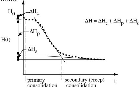
•The overall change in height of the specimen could be broken into three distinct contributions:
