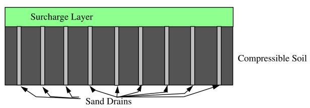
• With sand drains, the water in the compressible soil can flows to the nearest sand drain and then up into the surcharge layer. Since this greatly reduces the drainage distance through the impermeable compressible soil, it significantly reduces consolidation times.
