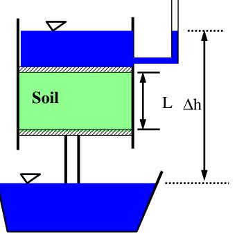
2. The Falling Head Test (relatively impermeable soils).
