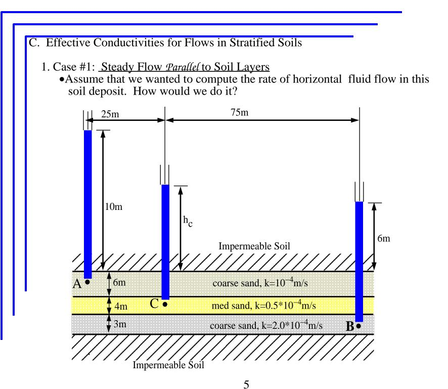
•Since the soil layers are bounded above and below by impermeable layers, the flow can only be parallel to the soil layers.
