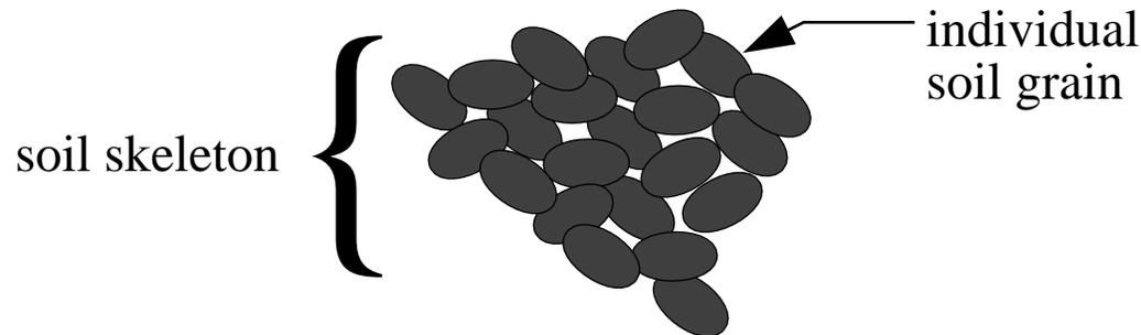
b) When loads are applied to the soil skeleton, deformations occur.
