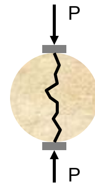
Fig. 11.6. Schematic of the split cylinder test.
