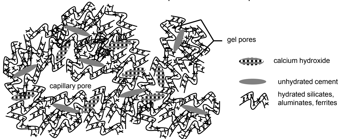
Fig. 9.3. Sketch of hcp microstructure showing the gel and capillary pores, the unhydrated cement, the calcium hydroxide, and the hydrated silicates, aluminates, and ferrites.
