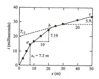
$$Z_1 = \frac{1}{2} \sqrt{\frac{v_2 - v_1}{v_2 + v_1}} x_c = \frac{1}{2} \sqrt{\frac{1390 - 492}{1390 + 492}} \times 7.5 = 2.6 \text{ m}$$
