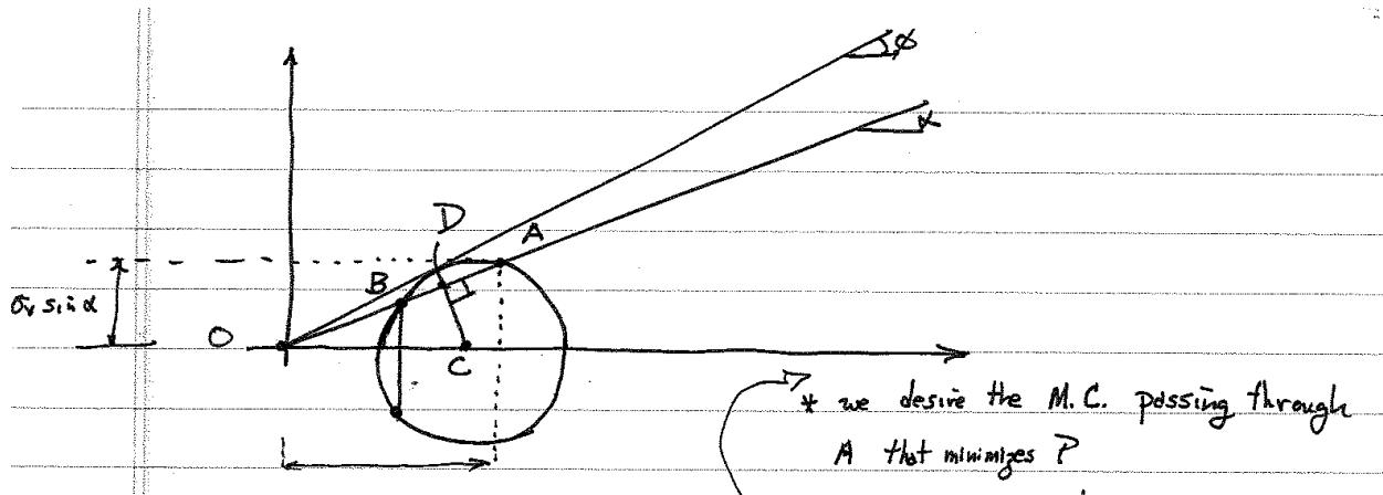
\* point A represents the stress state on planes  $\perp$  to the slope at depth  $z$
