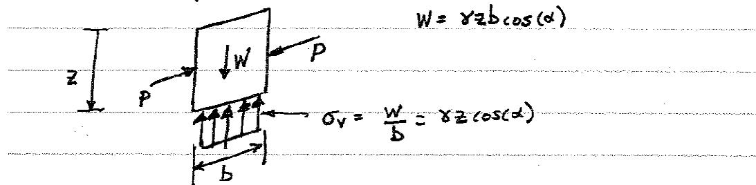
The force  $P$  is the ~~force~~<sup>one</sup> that would be exerted on a retaining wall, were one present.
