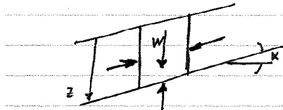
Isolating this slice from the slope and drawing its FBD we have:
