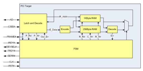
Figure 2 - Simple PCI Target with EDAC
