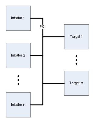
Figure 1 - PCI Bus System
