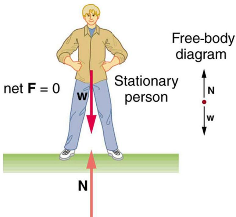
Figure 1: A simple and relatable example of static equilibrium (OpenSTAX, 2012).
