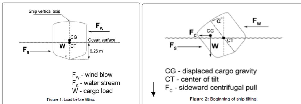
Figure 2: A visualization of the effects of the cargo's movement on the ship's equilibrium (Gorlov, 2014)
