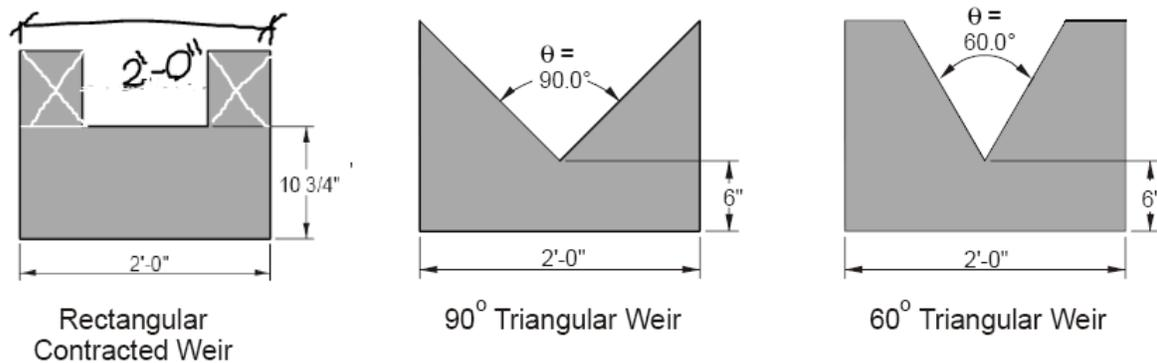
Figure 2. Geometry for typical weirs
