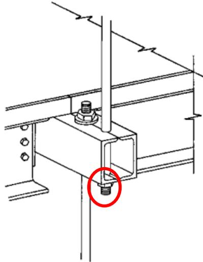
**Figure 2:** the support rod tore through the beam, causing the collapse of two walkways (Hyatt Regency Walkway Failure).
