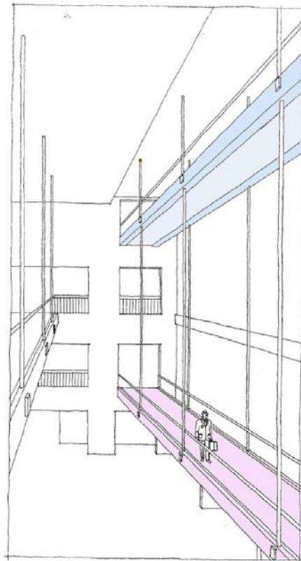
**Figure 1:** The design of the walkways placed the second and fourth walkways on the same support rods (Hyatt Regency Walkway Failure, 2014).
