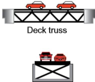
**Figure 2:** Representation of a Deck Truss Bridge
