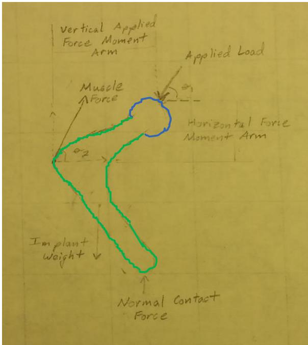
**Figure 2a.** A typical THR implant and the stresses acting on it
