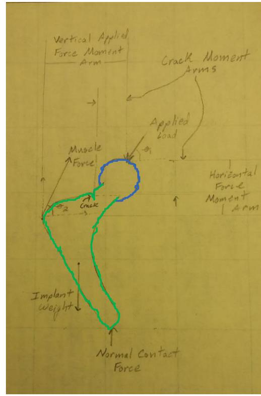
**Figure 2b.** A THR implant containing a crack in the upper femoral stem. This may lead to stress concentration and even device failure
