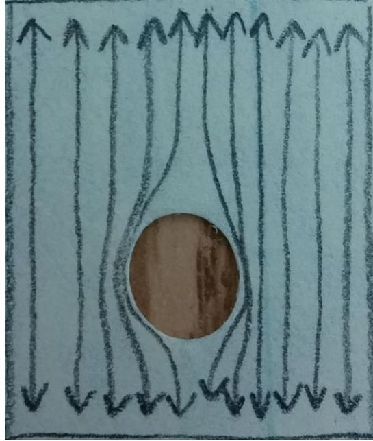
**Figure 1b.** A non-uniform object: stress is concentrated around the edges of the hole
